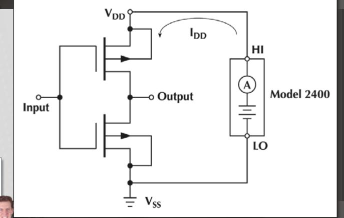
Measuring the quiescent current of a single CMOS inverter
