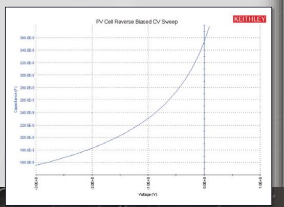
C-V sweep of a silicon solar cell
