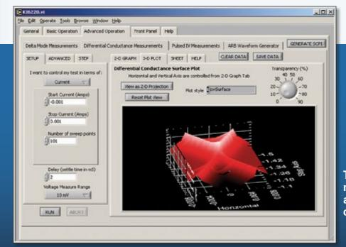
The 622X/2182A combination makes it simple to perform, analyze, and display differential conductance measurements. Download the Model 6220/6221 or Model 2182A data sheet.
