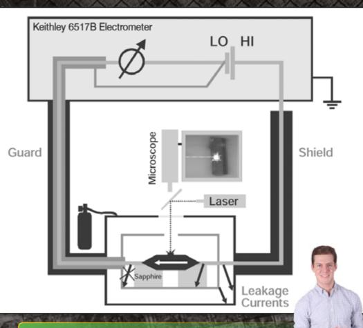
In this system configured for photocurrent measurements, the sample and the cable to the electrometer input are surrounded by a conductor at the same potential (guard) to prevent leakage currents.
