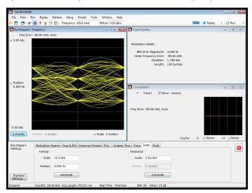
Option VM05 DECT, (2FSK 1.152 Mbps,1.925 GHz, 0 dBm), RMS FSK Err: 1.5%
