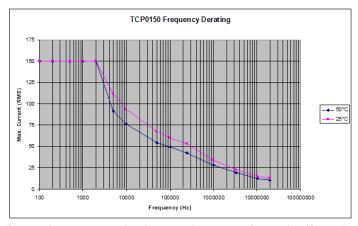
Do not apply currents greater than the max continuous current for more than 10 seconds to minimize heating effects.
