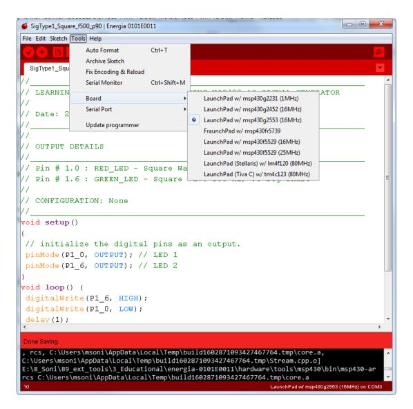
STEP: 6. Ensure that COM Port identified for your MSP430 Launchpad board is correct. You can also change / select appropriate COM Port your MSP430 Launchpad is connected as from following menu: Tools > Serial Port >
