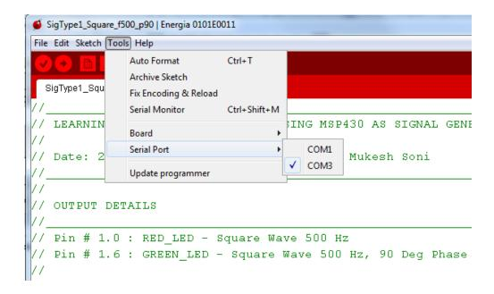
STEP: 7. Once the setting is complete, we are ready to download the program on MSP430 Launchpad board. We can test the setup by programming MSP430 Launchpad bard with an example code (sketch). Go to: File > Examples > 1.Basics > Blink
