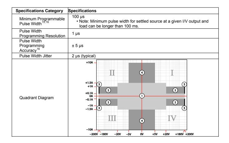
Typical performance for minimum settled pulse widths: Typical tests were performed using remote operation, 4W sense, and best fixed measurement range. For more information on pulse scripts, see the Series 2600A Reference Manual.
