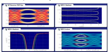
A key feature of the PAM-4 tool is to optimize the eye center reflecting a receiver with maximum horizontal and vertical margins. You have the option to lock the vertical slicer to a single phase for all three eyes.
