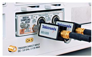
Sampling modules with dual electrical channels, such as the 80E04 dualchannel 20 GHz electrical sampling module with TDR, require two 80A09 devices. Step generators within the 80E04 TDR modules uses ≤ 250 mV. which is less than the diode threshold of the 80A09 device.
