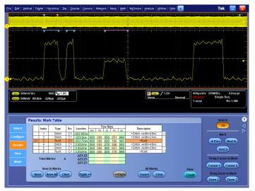
Search – Results of an advanced search for a runt pulse or a narrow glitch within a long waveform record. Each instance of the runt or glitch is automatically marked for easy reference. Wave Inspector controls provide unprecedented efficiency in viewing and navigating waveform data.
