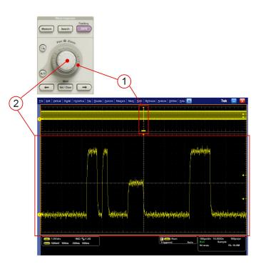
Wave Inspector controls provide unprecedented efficiency in viewing, navigating, and analyzing waveform data. Zip through your long record by turning the outer pan control (1). Get from the beginning to end in seconds. See something of interest and want to see more details? Just turn the inner zoom control (2).
