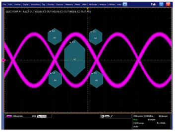
Eye Diagram triggering using optional Visual Trigger.
