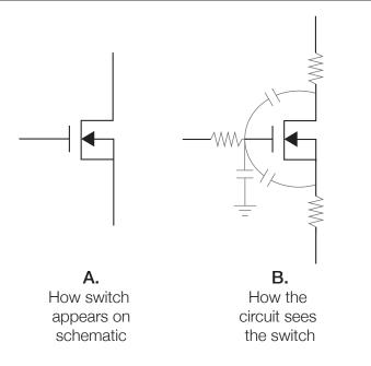
Figure 3. A: How the switch appears on the schematic, and  $\mbox{B:}$  How the circuit sees the switch.
