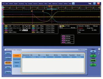
Figure 7. Automated slew rate measurement on MOSFET gate.
