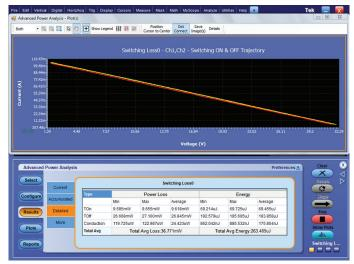
Figure 6. DPOPWR can show voltage versus current during turn-on (yello trace) and turn-off (red trace), over many cycles to see how characteristics change over time. The turn-on and the turn-off of this circuit are slow and balanced, so the plot is linear.
