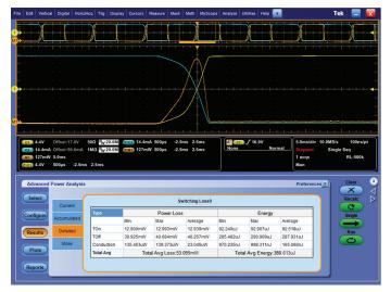
Figure 5. DPOPWR automated switching loss measurement.
