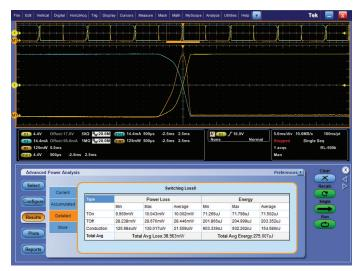
Figure 8. DPOPWR automated switching loss measurement, showing significant improvement.
