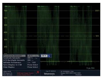
**Figure 8.** Note that the brightness of the trace is lower in one display than it is in the other. It is possible to control this with a menu setting at any time, but you can also program this brightness change into a preset that is accessible with the press of a button.
