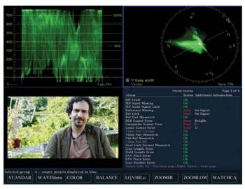
**Figure 5.** Note at the bottom of the screen that each preset has a customized name associated with a button. No need to scroll through menus to find a preset.
