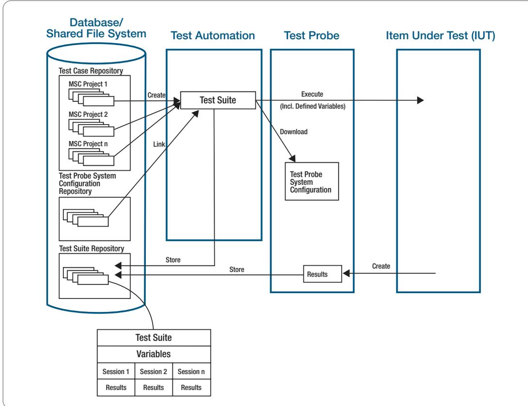
► **Figure 2.** The process of automated testing
