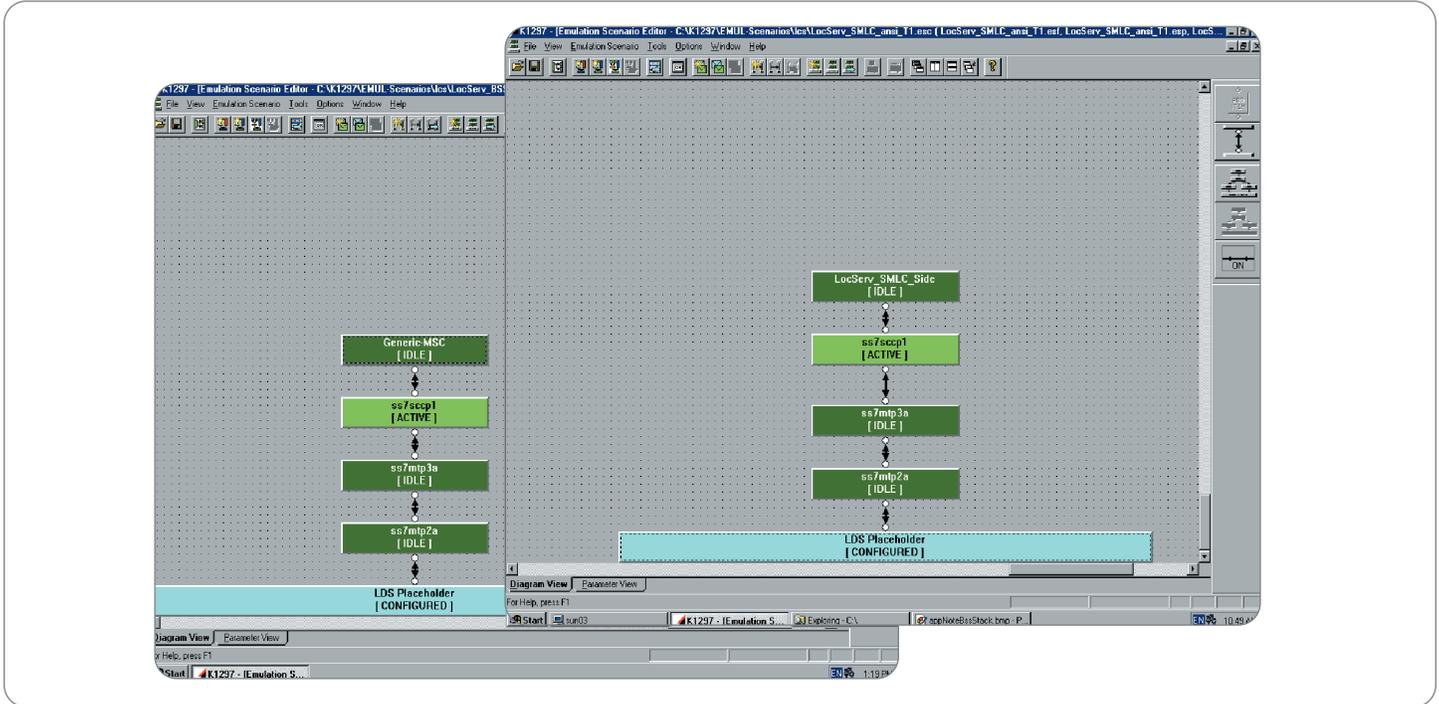
▶ **Figure 5.** Emulation stacks for the BSS and SMLC side
