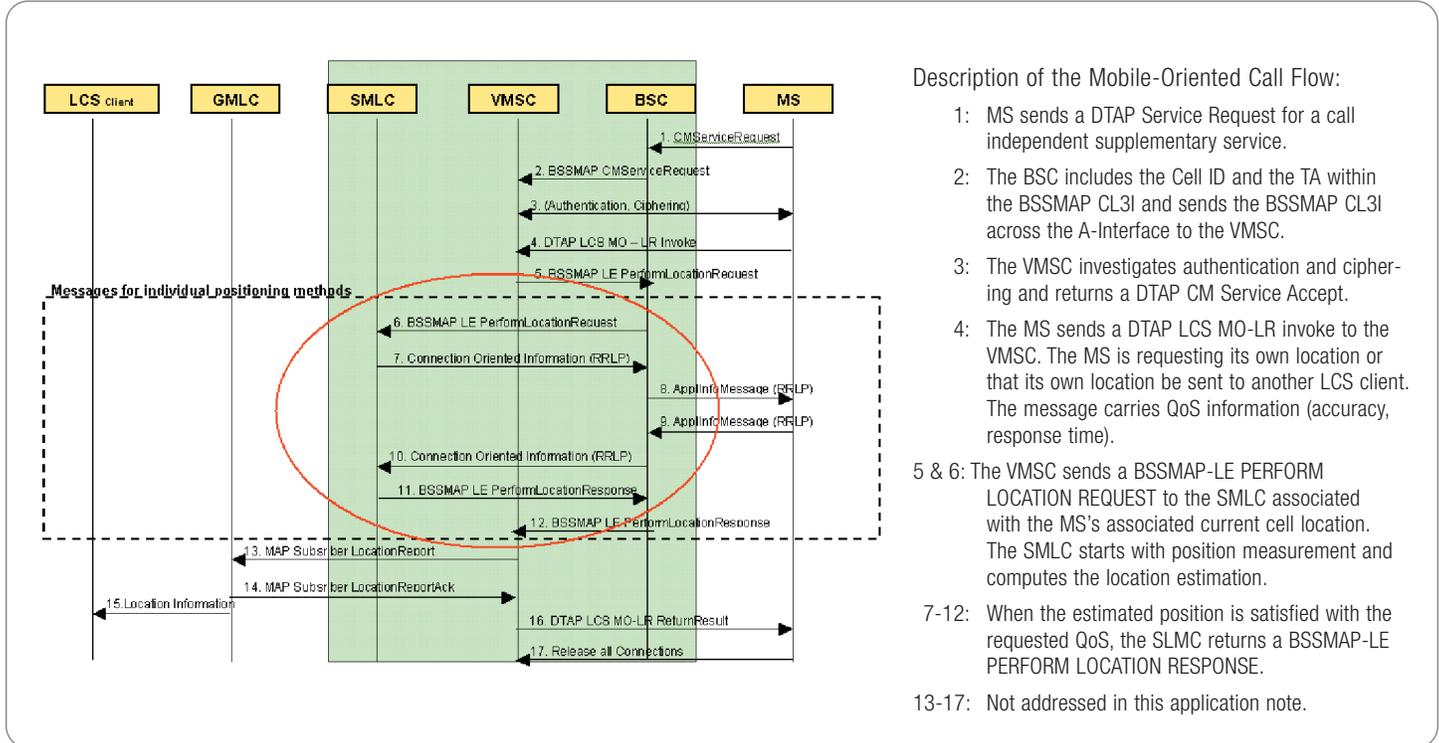
► **Figure 4.** Call flow of a mobile-oriented location request (BSS-based SMLC)
