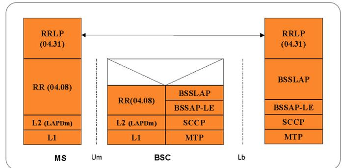
▶ **Figure 3.** BSS-based SMLC protocol stack
