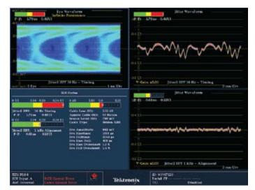
Figure 17. FlexVu<sup>™</sup> Physical Layer measurements.
