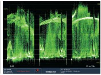
Figure 6. YRGB and RGB waveform displays.
