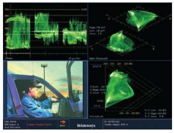
Figure 5. FlexVu<sup>™</sup> showing YPbPr waveform, Split-Diamond, Picture & Arrowhead displays.
