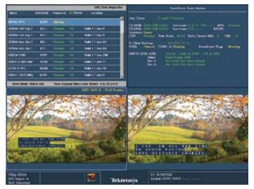
Figure 13. Simultaneous decode of 608 and 708 captions.
