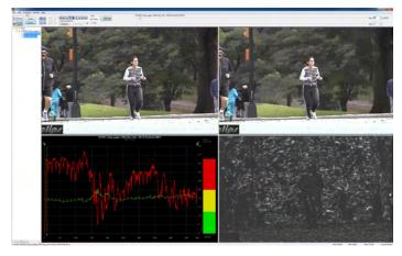
User Interface of PQA600. Showing reference, test sequences, with difference map and statistical graph.
