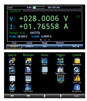
Figure 3. Adjust voltage, current, the current range, the measurement mode, protection levels, and other functions from the home screen.
