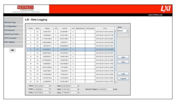
Figure 9. Web page display of the LXI-data logging function showing all parameters stored and the associated statistics.
