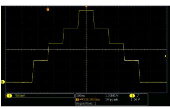
Figure 7B. Use the list mode to step the output voltage automatically through a series of levels. The voltages were created by the list shown in Fig. 7A.
