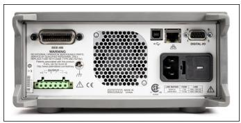
Figure 12. Series 2280S rear panel showing the rear output connector with remote sense inputs, digital I/O, and the three interfaces (GPIB, USB, and LAN).
