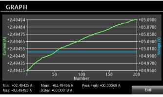
Figure 8. Monitor voltage, current, or both with the graphing function.
