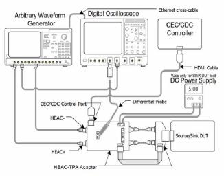
Setup 31. Test ID HEACT 5-16: Differential Signal Receiver Performance Test-Tektronix
