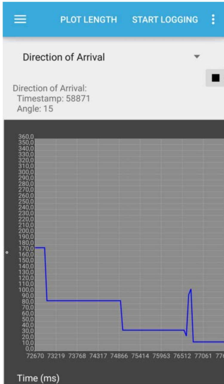
Figure 45. BlueMS (Android version) audio source localization plot example
