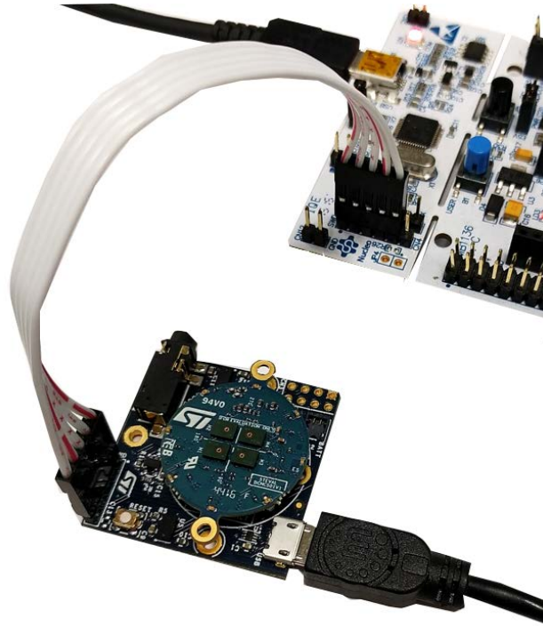
Figure 70. BlueCoin-STM32Nucleo: SWD connections with 5-pin flat cable
