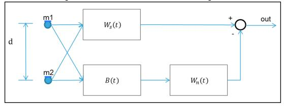
In the figure above, the  $W_s(t)$  operation implements the cardioid processing scheme shown in *Figure 7: "Optimization: Strong - block diagram"*, and operator implements a symmetrical schema where the microphones are exchanged so as to aim the beam in the opposite direction, with a 'zero' of the beam pattern towards the actual source. This configuration is known as back to back cardioid<sup>a</sup>.
