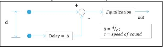
Figure 4: Cardioid basic block diagram
