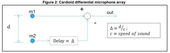
In an extended field context where all the acoustic sources are much further from the microphones than the distance "d" between microphones, the system can be described by the following equation:
