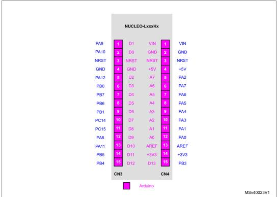
Figure 8. NUCLEO-L011K4, NUCLEO-L031K6, NUCLEO-L412KB and NUCLEO-L432KC pin assignment
