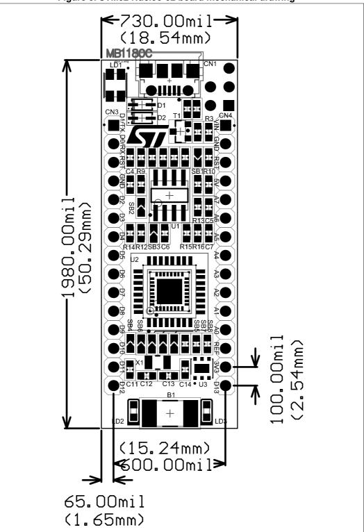
Figure 5. STM32 Nucleo-32 board mechanical drawing
