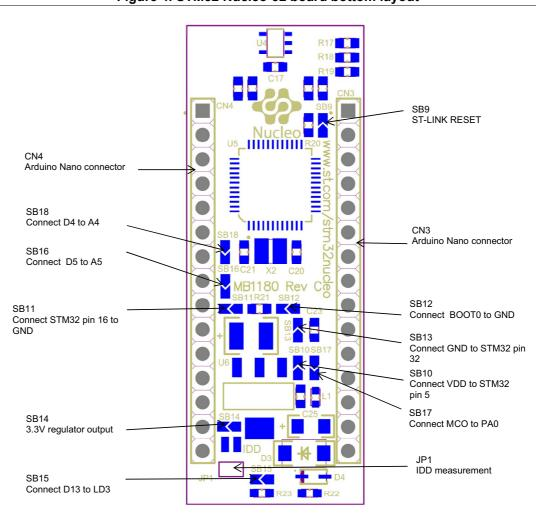
Figure 4. STM32 Nucleo-32 board bottom layout
