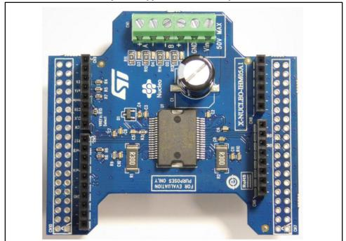
Figure 1: X-NUCLEO-IHM05A1 bipolar stepper motor driver expansion board based on the L6208
