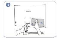
Grab the stand with one hand and use the thumb on your other hand to remove the COVER-REAR SUB in the direction of the arrow.
