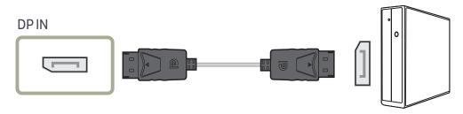
To display 3840 x 2160 @ 60 Hz, use a DP cable that supports 3840 x 2160 @ 60 Hz. Make sure that the graphics card of the DP source supports 3840 x 2160 @ 60 Hz.
