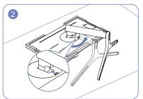
Push the key upward and hold. Turn the stand neck of the display counterclockwise for 10°.
