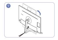
Rotate the machine to the horizontal position.
