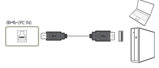
Connect the USB cable to  $\square$  on the back of the product and USB  $\square$  on the PC.
