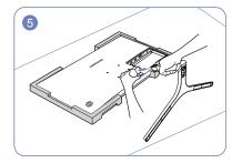
Hold the main body of the product with your hand as shown by the figure. Push the assembled stand into the main body in the direction of the arrow as shown in the figure.
