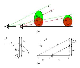
**Figure 7:** (a) Vertical distortion caused by capturing with cameras which lie on a larger circle than the ODS viewing circle. The red faces are viewed by a camera. When the parallel rays are used for rendering from a viewpoint behind the camera this leads to the vertically stretched green faces. (b) Top and side views of this distortion being applied to a point.
