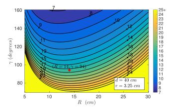
**Figure 10:** Minimum number of cameras as a function of rig radius R and horizontal field of view  $\gamma$ . The interpupillary distance is set to 6.5cm and the minimum distance d is set to 40cm. Increasing the number of cameras reduces field of view requirements while increasing the viewing circle radius increases the required field of view. The design choice in this work is shown as a large red dot at R = 14cm and  $\gamma = 94^{\circ}$ .
