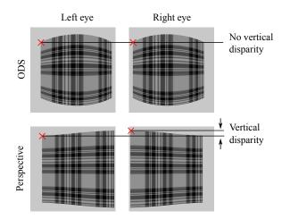
**Figure 3:** A synthesized, textured square imaged by the ODS projection and then projected to perspective. The images have an interpupillary distance of 6cm and about  $100^{\circ}$  FOV. The square has been placed at the unusually close distance of 30cm to exaggerate the vertical parallax for the figure.
