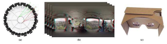
**Figure 1:** The Jump system produces omnidirectional stereo (ODS) video. (a) The multi-camera rig with the ODS viewing circle overlaid and three rays for the left (green) and right (red) stitches. Solid rays pass through a camera and can be sampled directly. Dashed rays are sampled from interpolated views. (b) A stitched ODS video generated from 16 input videos, shown in anaglyphic stereo here. (c) A VR headset in which the video can be viewed.
