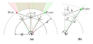
**Figure 9:** (a) To successfully stitch all points with distances of at least d from the rig center, the central camera must observe all points in the shaded regions (red for right eye and green for left eye). The extreme points  $p_{left}$  and  $p_{right}$  constrain the camera's field of view to be at least  $\gamma$ . (b) Here we visualize the intermediate values used when defining  $\gamma$  in (6).
