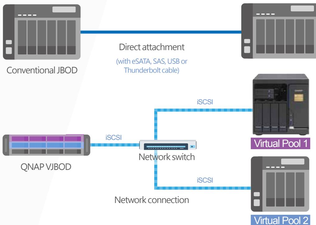
With the networked and virtual expansion units, online capacity expansion with all available space among multiple QNAP NAS is made possible in lieu of attaching a physical expansion unit. This also helps maximizing the utilization of storage resources.
