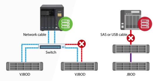
VJBOD + Port Trunking (offers connection fault tolerance)
