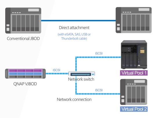
With the networked and virtual expansion units, online capacity expansion with all available space among multiple QNAP NAS is made possible in lieu of attaching a physical expansion unit. This also helps maximizing the utilization of storage resources.
