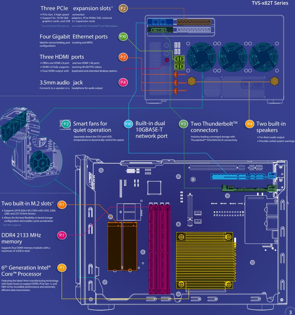
(P.9) Four built-in SSD 2.5" slots Offers flexible configuration in tiered storage and enables cache acceleration
