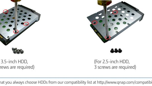
(For 3.5-inch HDD, 4 screws are required)
