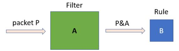
The packet enters the green filter which modifies it by masking it with the value A. The output value, P&A, is then compared to the value B, and if they are equal, then that is a match.
