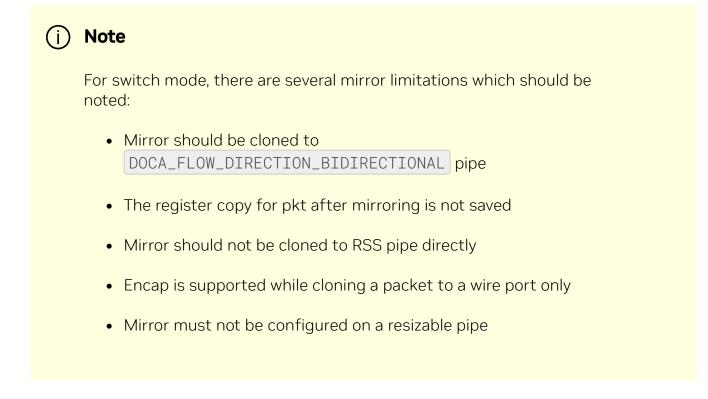
If mirror creation fails, users should check the resulting syndrome for failure details.
