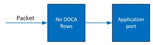
Once entries are added to the pipe, if a packet has no match then it continues to the port in the software. If it is matched, then the rules defined in the pipe are executed.
