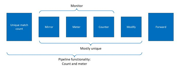
The creation phase allows the hardware to efficiently build the execution pipe. After the pipe is created, specific entries can be added. A subset of the pipe may be used (e.g., skipping the monitor completely, just using the counter, etc).
