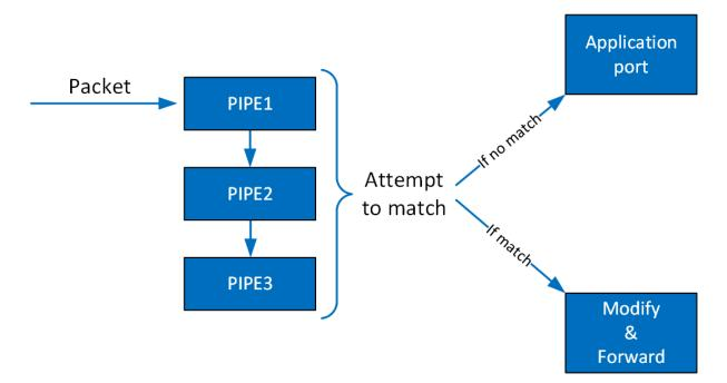
If the packet is forwarded in RSS, the packet is forwarded to software according to the RSS definition. If the packet is forwarded to a port, the packet is redirected back to the wire. If the packet is forwarded to the next pipe, then the software attempts to match it with the next pipe.
