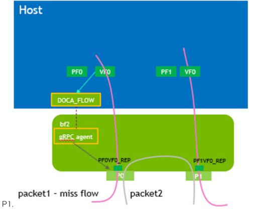
to set rules on PO, packet2 hits the rule, then is either dropped or is sent out from
