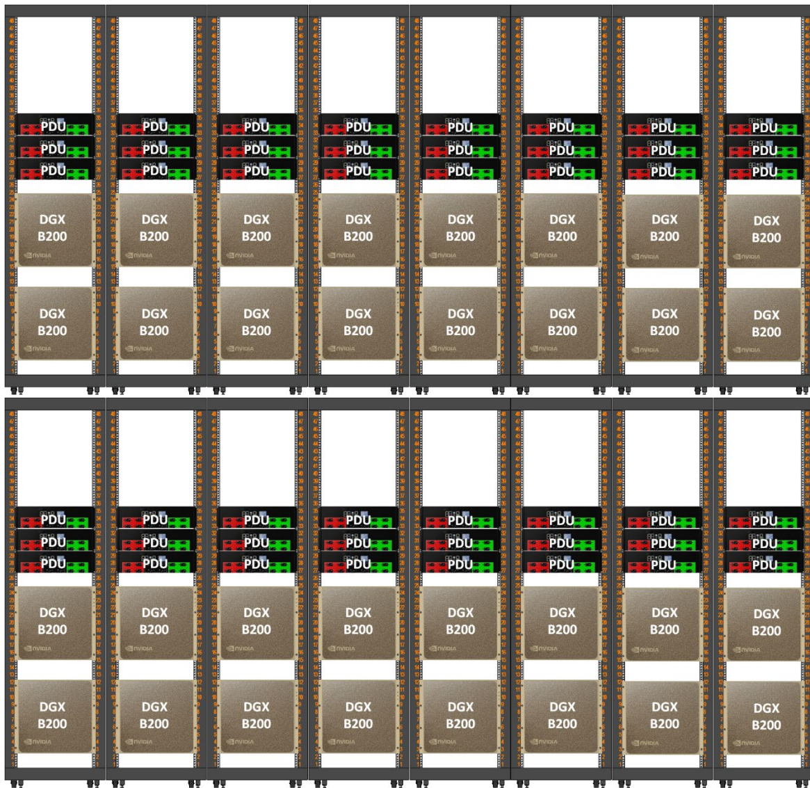
Figure 2. Complete single SU rack layout
