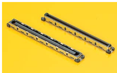
1. An integral metal shield and grounding tabs provide ESD protection and pc-board retention on high circuit-size board-to-board connectors. (courtesy of Molex)
