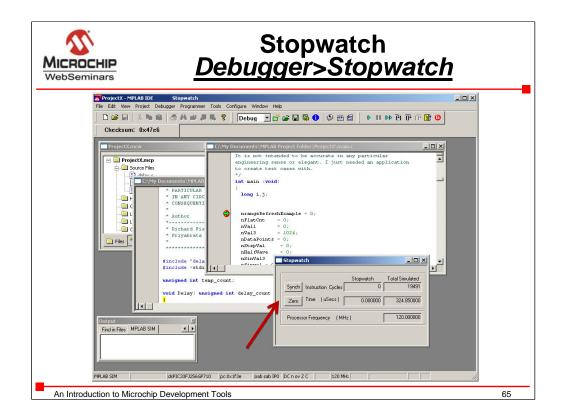
MPLAB SIM has tools to analyze how the code is running.
