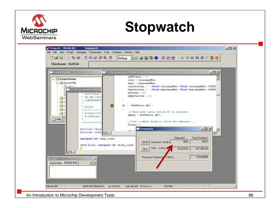
Run to the next breakpoint, and the stopwatch accurately measures the instruction time in cycles and microseconds.
