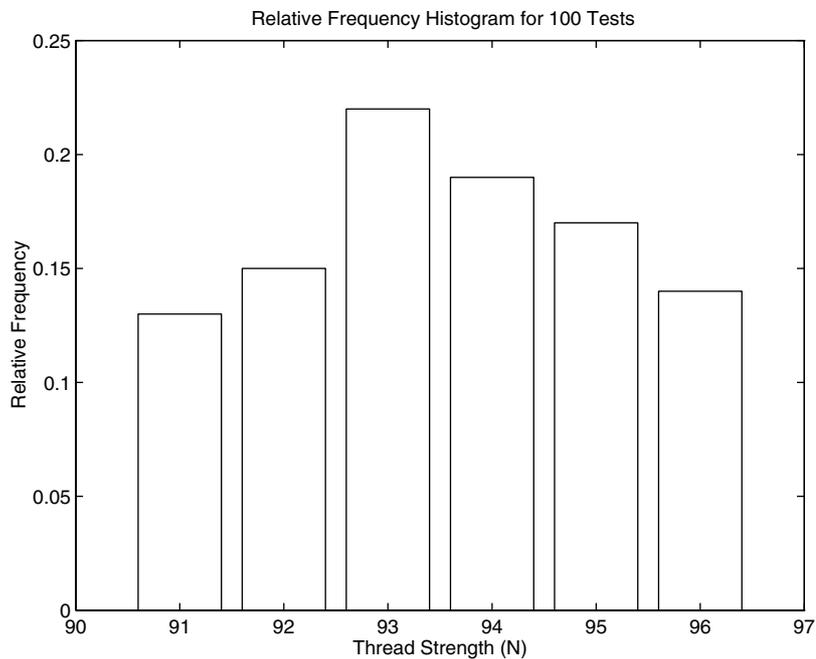
**Figure 7.1–3** Relative frequency histogram for 100 thread tests.
