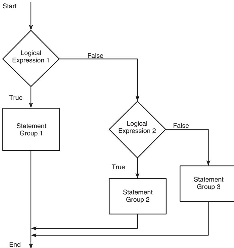
**Figure 4.4–3** Flowchart for the general `if` structure.
