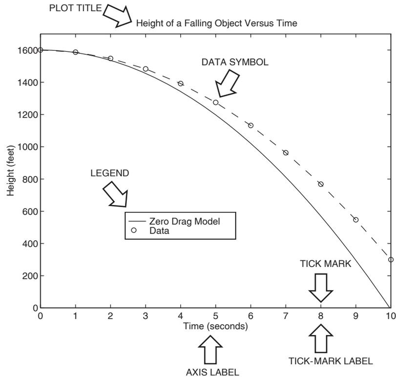
Figure 5.1-1 Nomenclature for a typical  $xy$  plot.
