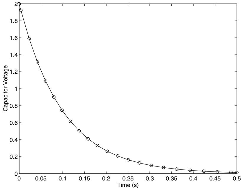
**Figure 9.3-2** Free response of an  $RC$  circuit.
