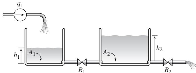
Figure 10.7-5 A hydraulic system with two tanks.
