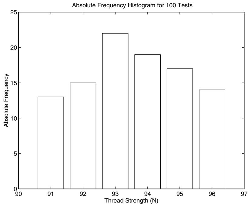
Figure 7.1–2 Absolute frequency histogram for 100 thread tests.
