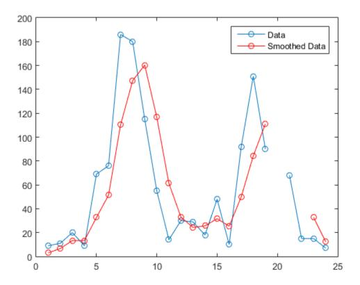
The smoothed data are shifted from the previous plot. **convn** with the '**same**' parameter returns the central part of the convolution, the same length as the data. filter returns
