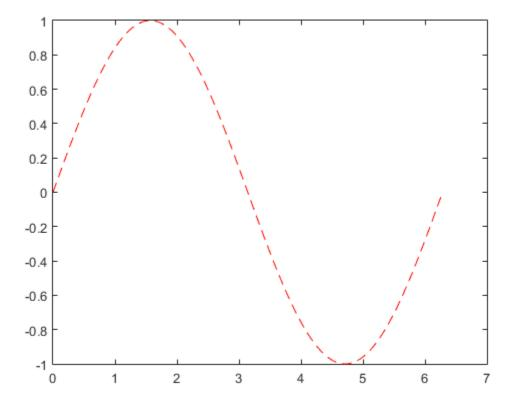
The 'r--' string is a *line specification*. Each specification can include characters for the line color, style, and marker. A marker is a symbol that appears at each plotted data point, such as a +, 0, or \*. For example, 'g:\*' requests a dotted green line with \* markers.
