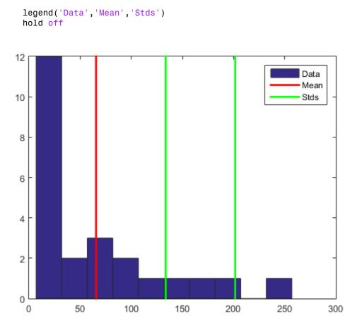
The plot shows that some of the data are more than two standard deviations above the mean. If you identify these data as errors (not features), replace them with NaN values as follows:
