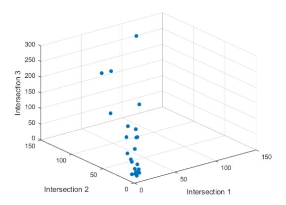
Measure the strength of the linear relationship among the variables in the threedimensional scatter by computing eigenvalues of the covariance matrix with the **eig** function:
