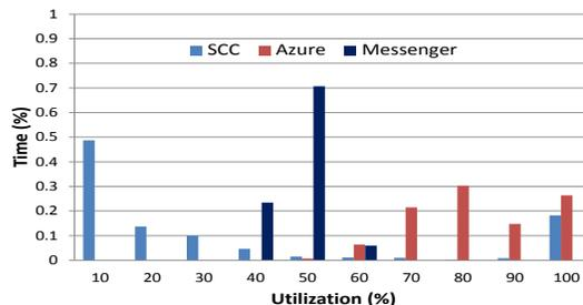
**Fig. 3:** Cluster utilization histogram for the three traces. For the SCC trace, the fraction of active servers is below 30% half of the time but is 100% utilized about 20% of the time. The Messenger and Azure clusters have about 50% utilization and about 80% utilization 70% of the time, respectively, with high load variation.
