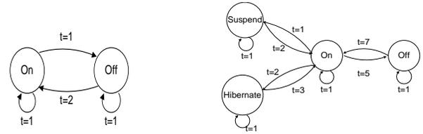
**Fig. 4:** Markov state diagram of transitions for (a) On-Off and (b) On-Off-Suspend-Hibernate power schemes. In the On-Off state diagram, the system can transition from On to Off in one time step and from Off to On in two time steps.
