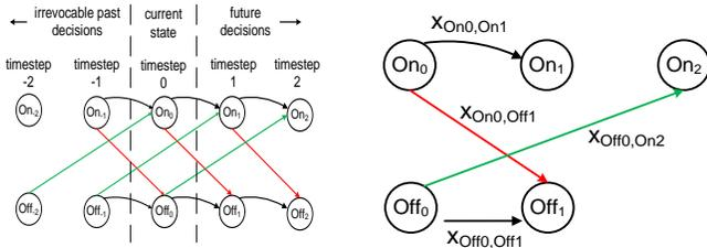
**Fig. 6:** (a) State diagram unrolled in time. If the timestamp of an edge is less than zero it cannot affect the current state or future decisions; these edges are not shown. For the On-Off system no states occurring earlier than time step -2 can affect the current state; these states are not shown. (b) Edge labeling convention.
