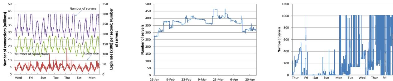
**Fig. 1:** Load patterns for the (a) Messenger, (b) Azure, and (c) SCC traces. We observe highly periodic nature of Messenger, small load variation for Azure, and a high dynamic range and sharp transient spikes for the SCC trace.
