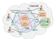
Figure 1: High-level architecture of many CDNs.
