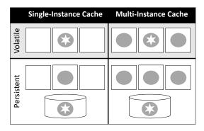
Fig. 2. The four actor configuration options in a multi-cluster. Squares are clusters, Cylinders are the storage layer, circles are copies of the actor state, and the star marks the latest version (primary copy).
