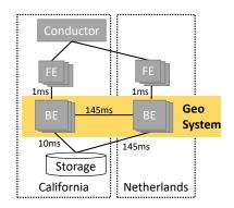
Fig. 7. Setup and approximate round-trip times.
