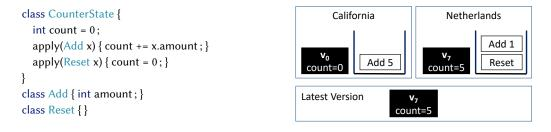
Fig. 4. (a) **left**: example definition of state and update objects. (b) **right**: sample snapshot of the internal state of an actor that uses the versioned state API and has two instances in different datacenters.
