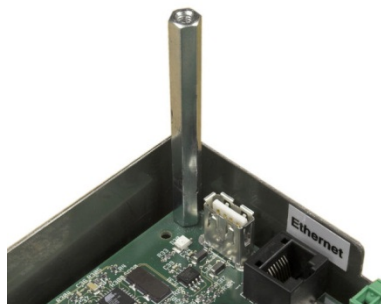
Figure 3-53: Stand-Off on Main PCB
