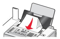
2 Adjust the paper guides on the ADF to rest against the edges of the paper.
