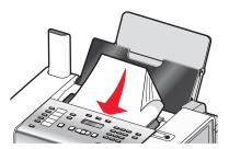
2 Adjust the paper guides on the ADF to rest against the edges of the paper.
