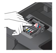
**Note:** Install the new ink cartridges immediately after removing the protective cap to avoid exposing the ink to air.
