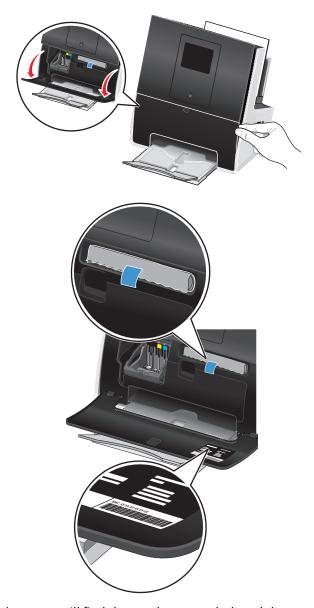
Behind the printhead access door, you will find the touch-screen cloth and the customer support label, which identifies the model number of the printer, the customer support hot line, the ink cartridge information, and the MAC address.
