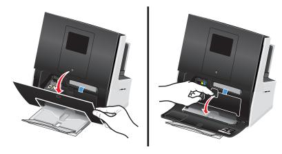
**2** Pull the latch forward, and then remove the printhead.
