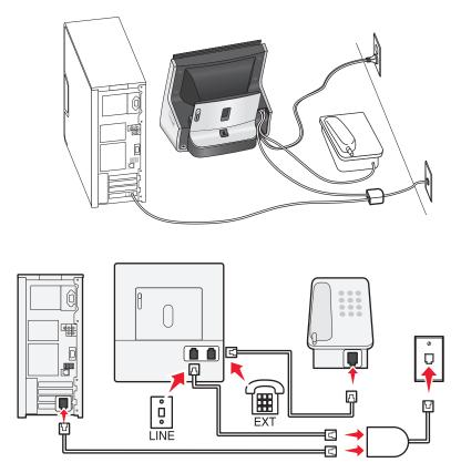
A Digital Subscriber Line splits your regular telephone line into two channels: voice and Internet. Telephone and fax signals travel through the voice channel, and Internet signals pass through the other channel. This way, you can use the same line for analog voice calls (including faxes) and digital Internet access.
