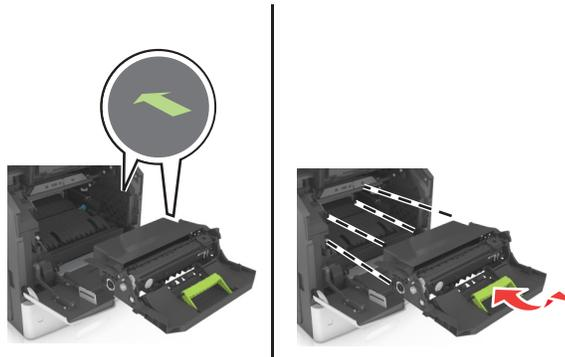
**7** Insert the toner cartridge into the printer by aligning the side rails of the cartridge with the arrows on the side rails inside the printer.
