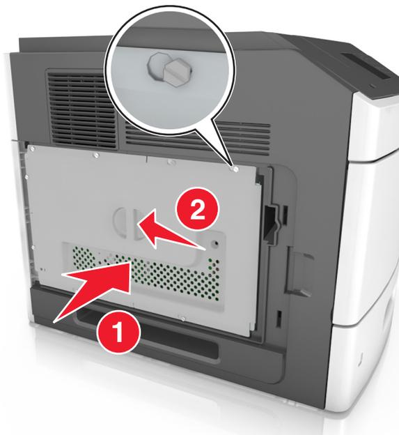
6 Tighten the screws on the shield.
