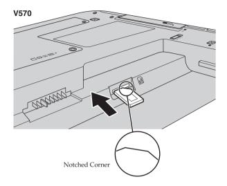
**5** Put the battery back in place. Turn the computer over and reconnect the cables.
