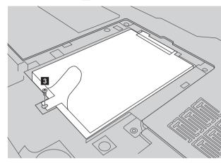
**5** Remove the frame fixing screw **3**.
