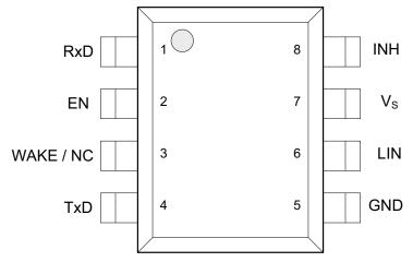
Figure 1 Pin-out of standard 8-pin LIN transceiver
