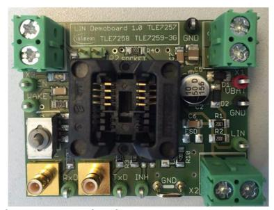
Figure 2 Photo of the DSO-8 LIN Demoboard
