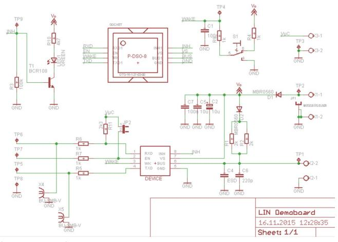
Figure 3 Schematic of DSO-8 LIN Demoboard
