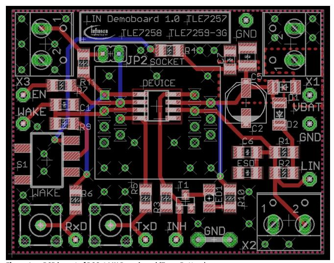
Figure 4 PCB layout of DSO-8 LIN Demoboard (Top + Bottom)
