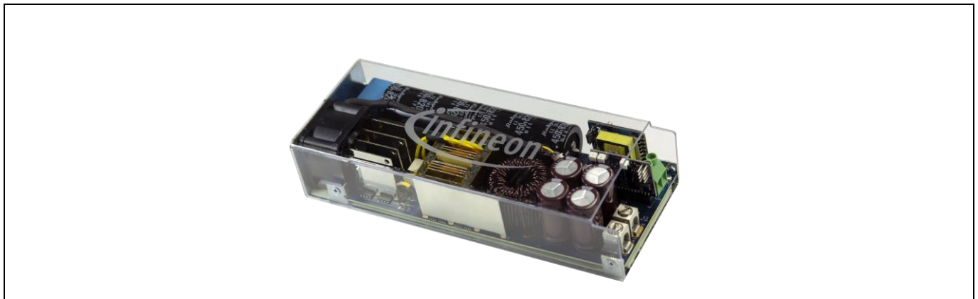
Figure 1 3300 W bi-directional PSFB
