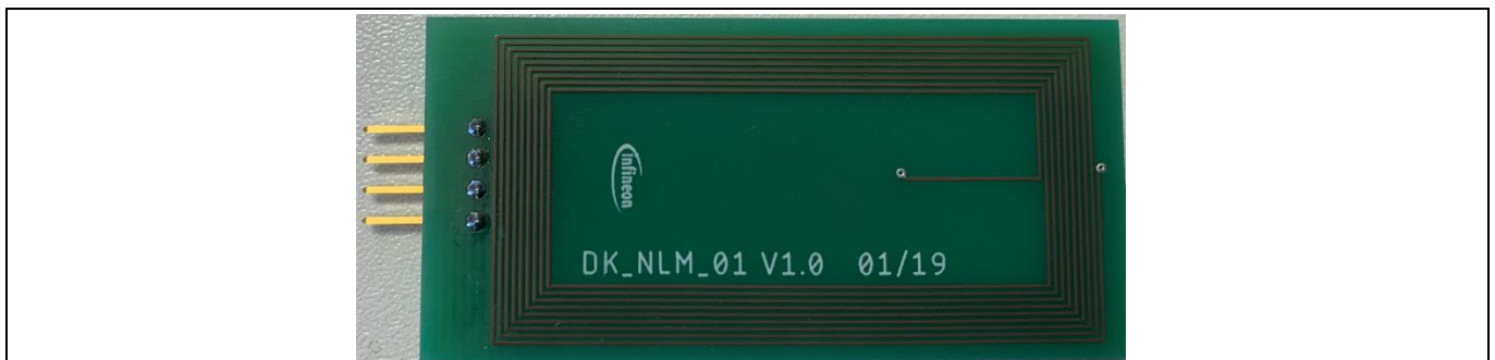
Figure 14 Top view of DK_NLM_01 with NFC antenna
