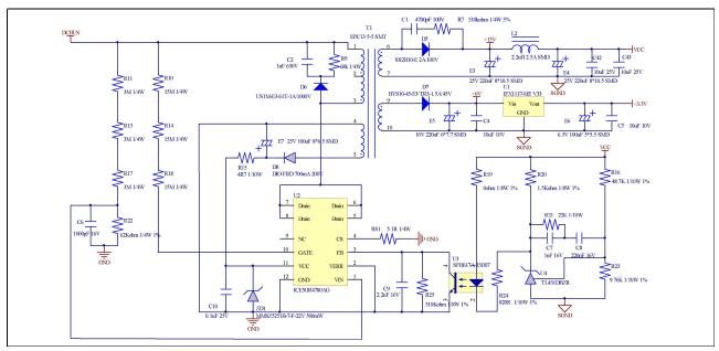
Power supply section of the EVAL-C101T-IM231 evaluation board Figure 16
