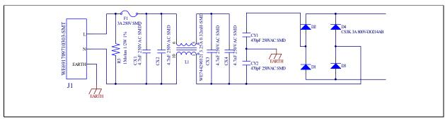
Figure 13 The schematic for AC/DC section and EMI of the EVAL-C101T-IM231 evaluation board
