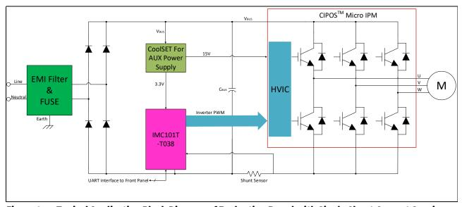
Figure 2 Typical Application Block Diagram of Evaluation Board with Single Shunt Current Sensing
