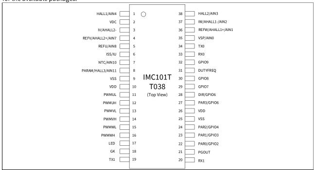
Figure 3 Pinout of IMC101T-T038
