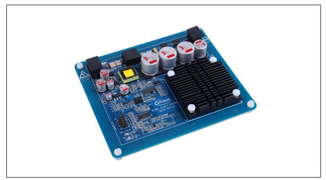
Figure 1 Evaluation board of the EVAL-C101T-IM231
