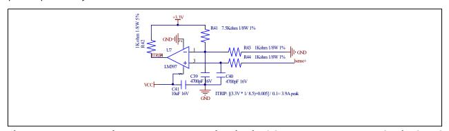
Figure 17 Inverter section over current protection circuit of the EVAL-C101T-IM231 evaluation board
