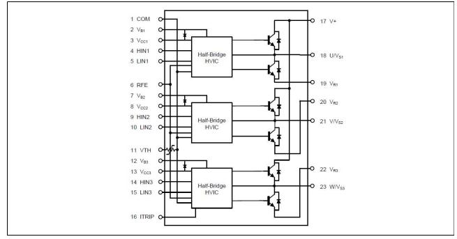
Figure 4 Internal electrical schematic
