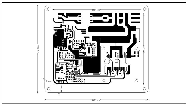
Figure 20 Top layer routing of the EVAL-C101T-IM231
