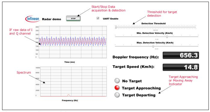
Figure 21 Data display on Micrium GUI
