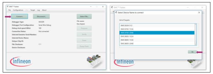
Figure 9 XMC<sup>™</sup> Flasher device selection and connection
