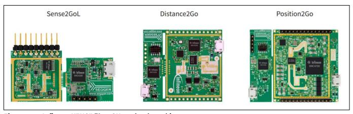
Figure 1 Infineon XENSIV™ 24 GHz radar demo kits
