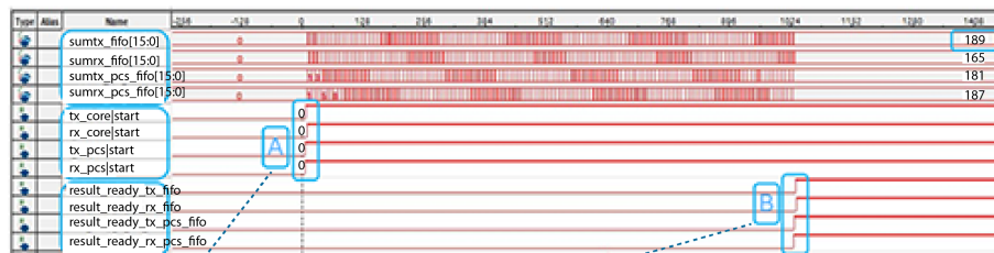
Figure 88. FIFO Latency Calculation Logic for Four FIFOs
