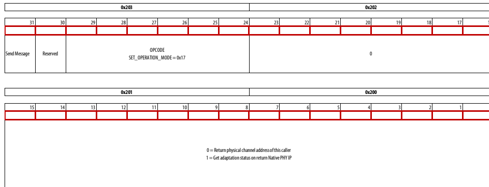
Figure 118. Loading PMA Configuration Register CHECK_CAL_STAT
