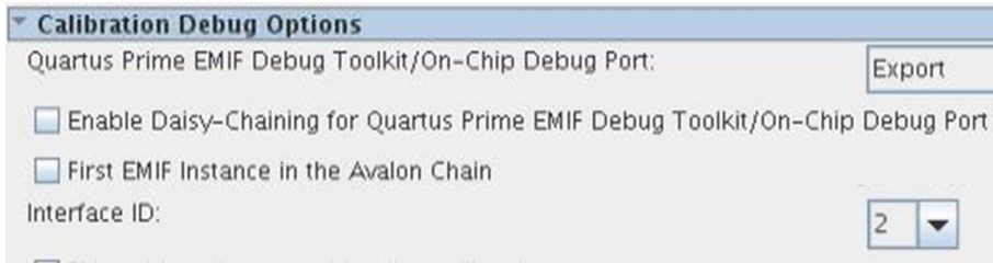
Figure 114. EMIF with EMIF Debug Interface Exported and Daisy-Chain Disabled
