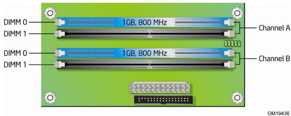
Figure 13. Dual Channel Memory Configuration Example 1
