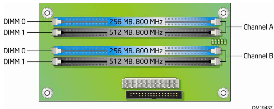
Figure 14. Dual Channel Memory Configuration Example 2
