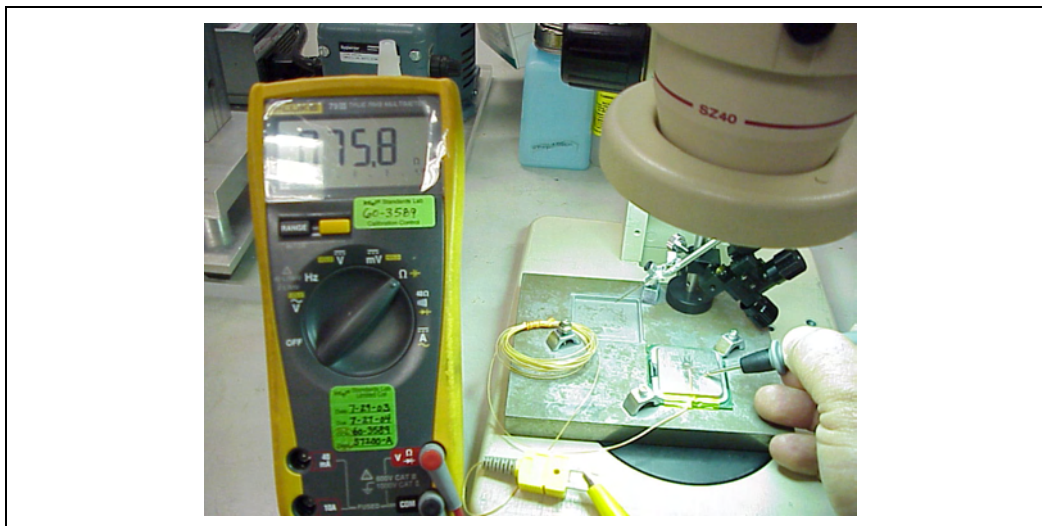
Figure 37. Applying the Adhesive on the Thermocouple Bead
