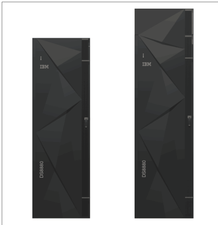
Figure 1-1 DS8884 40U Rack and the expanded DS8886/DS8888 46U Rack
